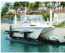
AirBerth is suitable for both mono hull planning and catamaran style hulls
