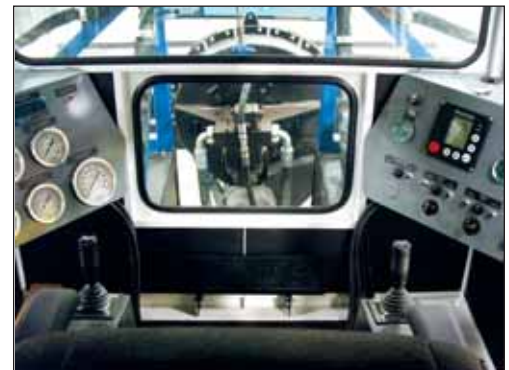
All Versi-Dredge® models come standard with joystick controls and oversized gauges for ease of operation.
